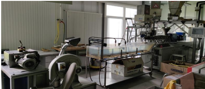
Fig: Double screw extruder used for compounding process
